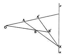
and let A' be the point corresponding to the point A. Let B be any other point of F, B' the corresponding point of F'. Then since AB, A'B' are corresponding lines, they must intersect on the axis x. Let AB cut the axis x in the point X. Then A'X will intersect OB in required point B'. In the same way the point corresponding to any other point may be constructed.
